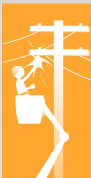
**NEVER** connect generators directly to household wiring without first installing a **TRANSFER SWITCH**. This prevents backfeeding which could electrocute utility workers making repairs.
