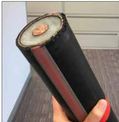
One phase of the 115kV transmission line
