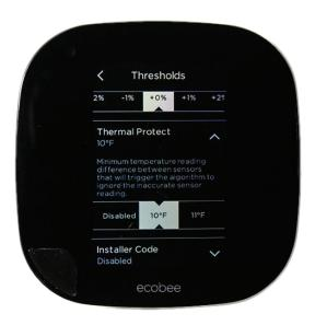
This maximizes system efficiency and minimizes a situation where a poorly located sensor may throw off thermostat functionality.
