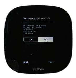
Verify that your system is wired to maximize its capabilities and work best with the new thermostat. If accessories are installed, identify what is installed and reference the ecobee<sub>3</sub> installation documents to promote optimal performance.
