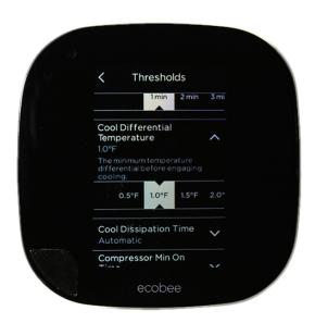
A 74°F set point will turn the cooling on at 75°F. Selecting 0.5°F may increase energy usage and reduce durability of system through more frequent on-off cycles, as compared to 1.0°F or higher.
