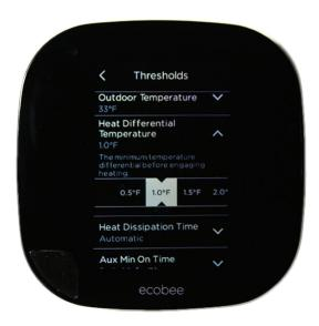
A 71°F set point will turn the heat on at 70°F. Selecting 0.5°F may increase energy usage and reduce durability of system through more frequent on-off cycles, as compared to 1.0°F or higher.
