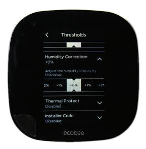
Leaving this setting at 0% does not adjust what humidity the thermostat displays versus what it actually is.
