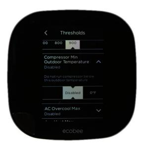
This maximizes efficiency of your air source heat pump before less efficient strip heat comes on to maintain comfort at lower temperatures.
