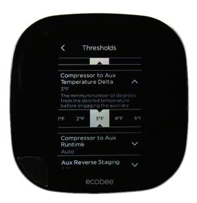
This is to maximize efficiency of your air source heat pump before less efficient strip heat comes on to maintain comfort at lower temps.
