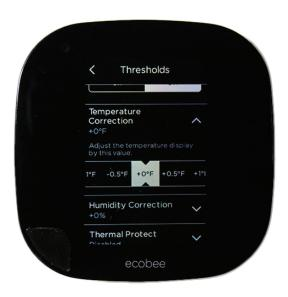
Leaving this setting at 0°F does not adjust what temperature the thermostat displays versus what it actually is. If you want to adjust the temperature displayed, you can do so with this setting.
