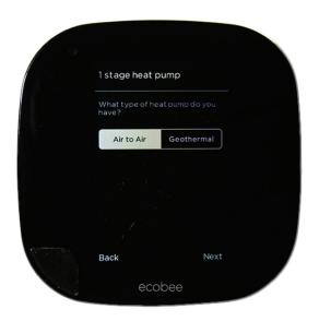
These are the recommended settings for a single-stage all electric air to air heat pump. See ecobee<sub>3</sub> installation documents if any other source of heating (e.g. water, propane, natural gas, etc.) is present.
