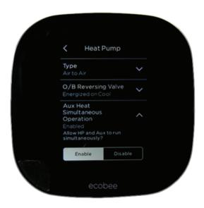
This is the recommended setting to maximize efficiency of your air source heat pump before less efficient strip heat comes on to maintain comfort at lower temps.
