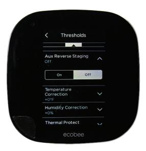
This is to maximize efficiency of your air source heat pump when less efficient strip heat comes on to maintain comfort at lower temps.
