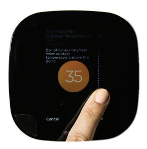
This temperature range is recommended to maximize efficiency of air source heat pump before less efficient strip heat comes on to maintain comfort at lower temperatures
