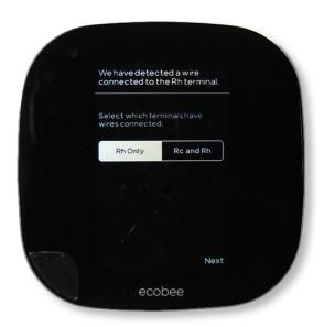
Select RH Only when your HVAC system has only one transformer to control it. If your system has two transformers installed, you should select Rc and Rh
