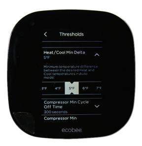
This promotes a long-lasting system and minimizes times when the system could bounce back and forth between cooling and heating, consuming more energy than desired.
