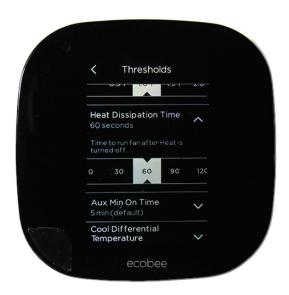
Sixty seconds will maximize the distribution of remaining heat in the system, but not circulate cool air if set for longer.
