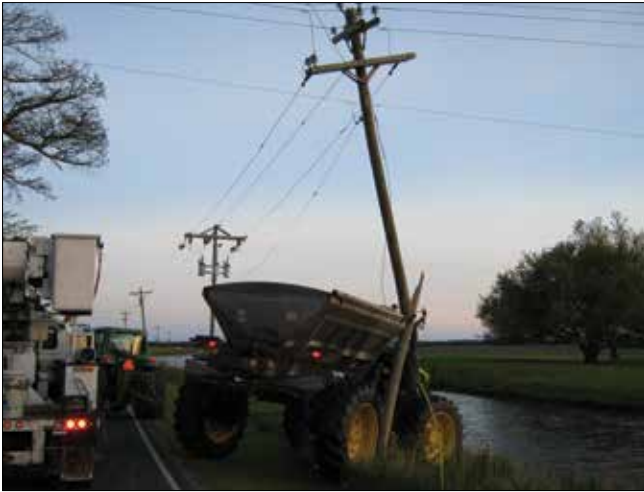
On April 11, a lime spreader narrowly missed going into a Hyde County canal when a broken hydraulic line resulted in a loss of steering. (Photo by Andy Midyette)
