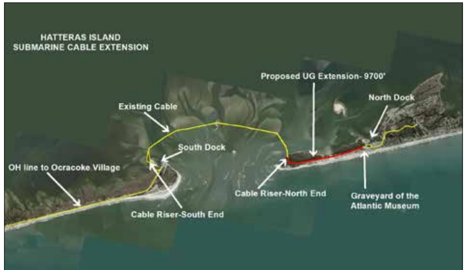
The new cable is represented in red in the image above. Tideland EMC operations department graphic
