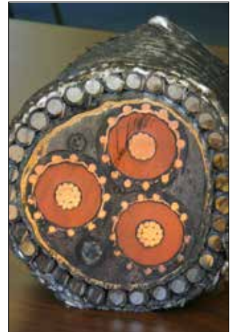
A cross section of the armored cable. Kim Fennema photo
