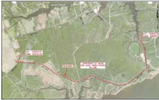
The engineer's rendering of the eventual tie-line for the Merritt and Dawson Creek circuits
