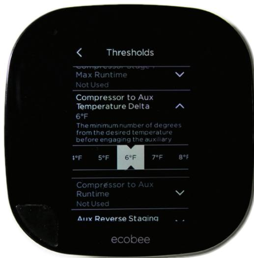
This is to maximize efficiency of your air source heat pump before less efficient strip heat comes on to maintain comfort at lower temps.
