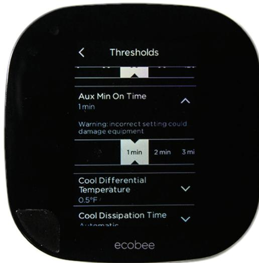
This setting regulates the electric heat run time which maximizes energy savings and increases durability of the system.
