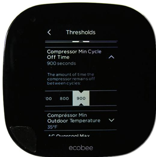
This is a recommended setting to save energy and increase equipment durability. After the unit cycles off, it will not come back on for 15 minutes.
