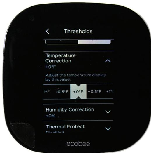
Leaving this setting at 0°F does not adjust what temperature the thermostat displays versus what it actually is. If you want to adjust the temperature displayed, you can do so with this setting.
