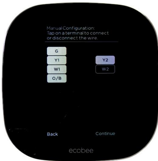
Verify that your system is wired to maximize its capabilities and work best with the new thermostat.
