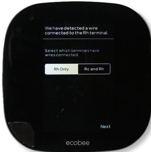
Select RH Only when your HVAC system has only one transformer to control it.
