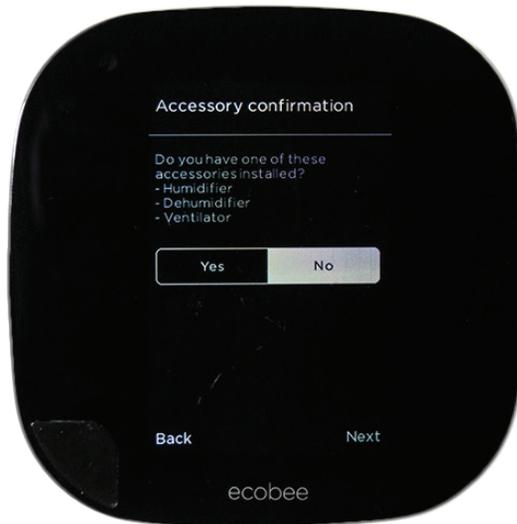
Verify that your system is wired to maximize its capabilities and work best with the new thermostat. If accessories are installed, identify what is installed and reference the ecobee<sub>3</sub> installation documents to promote optimal performance.
