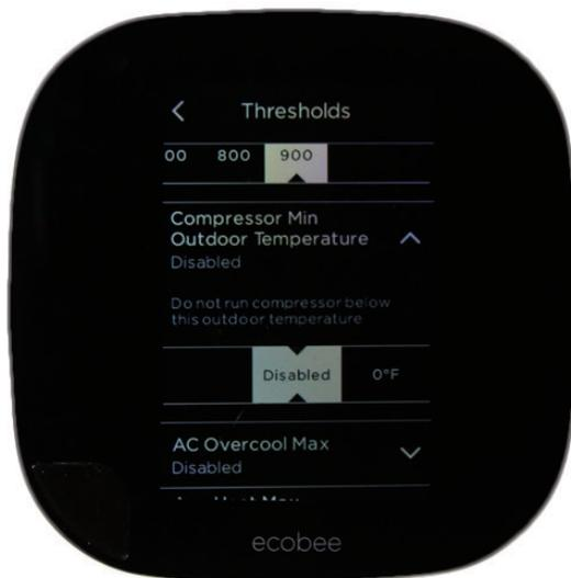
To maximize efficiency of your air source heat pump before less efficient strip heat comes on to maintain comfort at lower temperatures.
