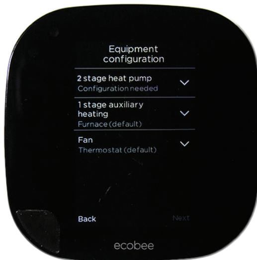
Auxiliary heating is a less efficient heating mode your air source heat pump may use at lower outdoor temperatures.
